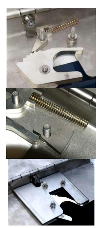
Ensure that the lock claw and pawl are free to move. The nuts want to be tight enough not to rattle, but loose enough to allow free movement.
