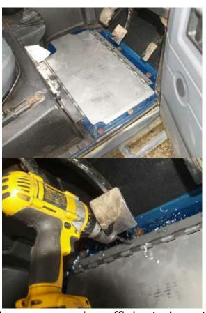
holes due to clearance issues. A minimum of three screws is sufficient. Insert screws into the holes with washers, then screw on a security nut & washer on to each. The hexagonal portion of the nut must face downwards. Make sure you are happy with its operation before you fully tighten.
